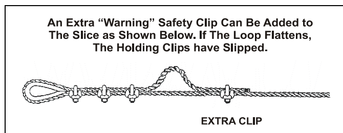
Figure 3-5. Joining Wire Ropes.
