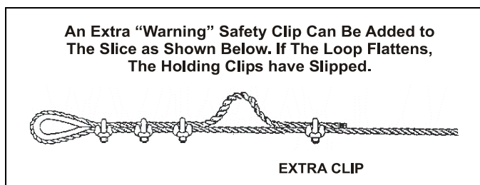
Figure 3-5. Joining Wire Ropes.
