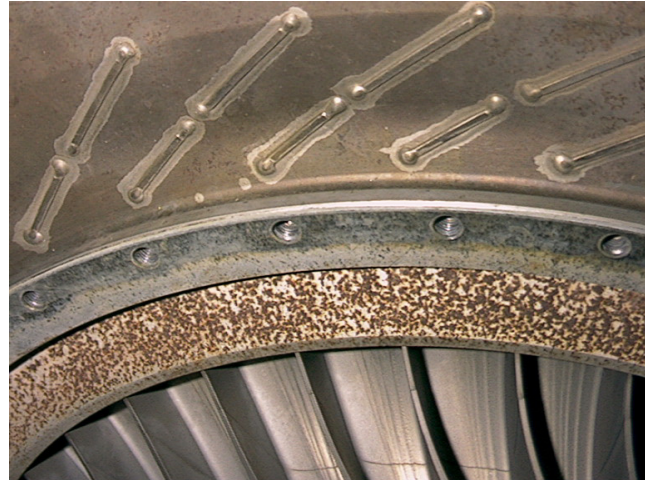
Figure 3-22. Hot Corrosion on Engine Components
