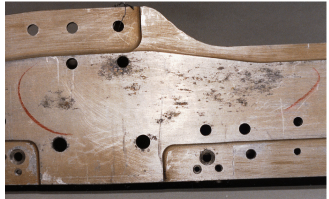
Figure 3-10. Pitting of an Aluminum Wing Assembly
