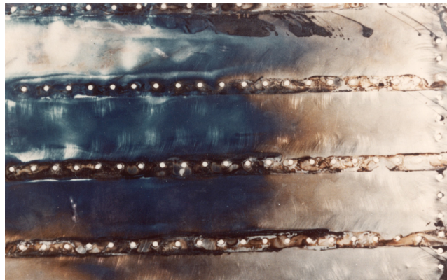
Figure 3-26. Color Changes in Titanium Due to Heating
