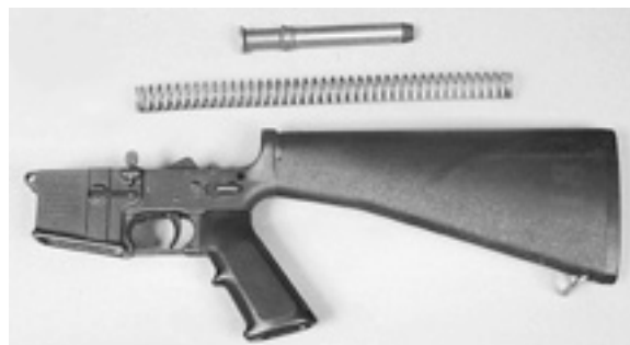
Figure 2-18. Lower Receiver Disassembled.
