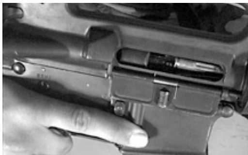
Figure 3-15. Brass Obstructing the Chamber.
