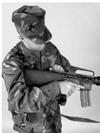
Figure 7-1. Pulling Charging Handle with Left Hand.
