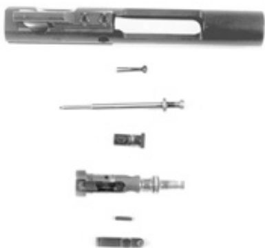
Figure 2-17. Bolt Carrier Disassembled.
