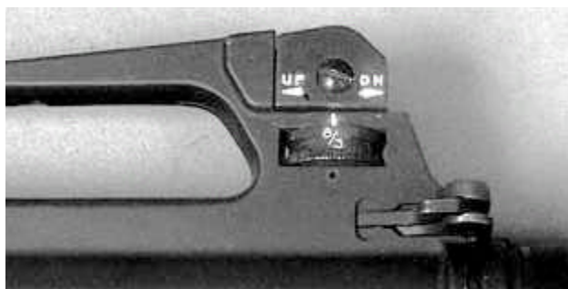
Figure 9-6. Rear Sight Elevation Knob Set for 300 Yards/Meters.
