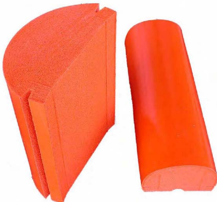
Figure 1: Ionomer Foam Collar Cross-Section Currently in use on the RB-M
