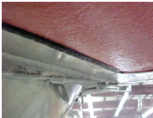
Figures 2 & 3: Current configuration of RB-S Collar/Fin interface, showing installation and details of Adhesive seal between the collar and Lower Flange.
