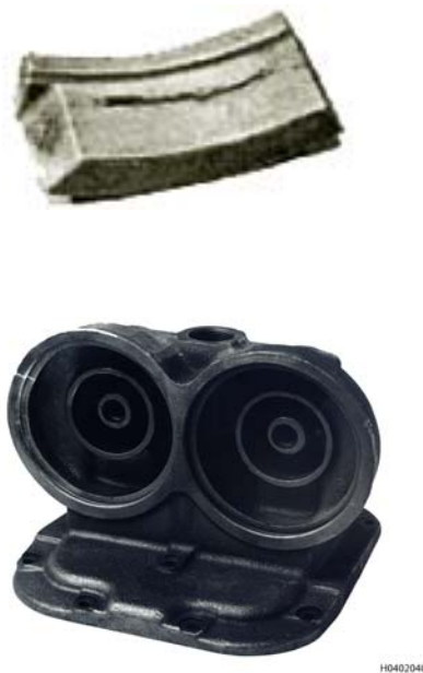
Figure 3-59. Magnetic Particle Indications of Defects in Castings
