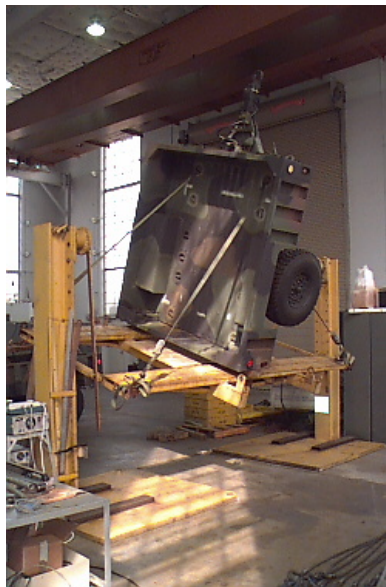
Figure 6: Yaw Moment of Inertia Measurement of Entire Trailer
