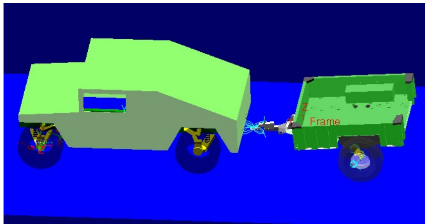
Figure 3: Combined Vehicle and Trailer Multi-body Dynamics Model
