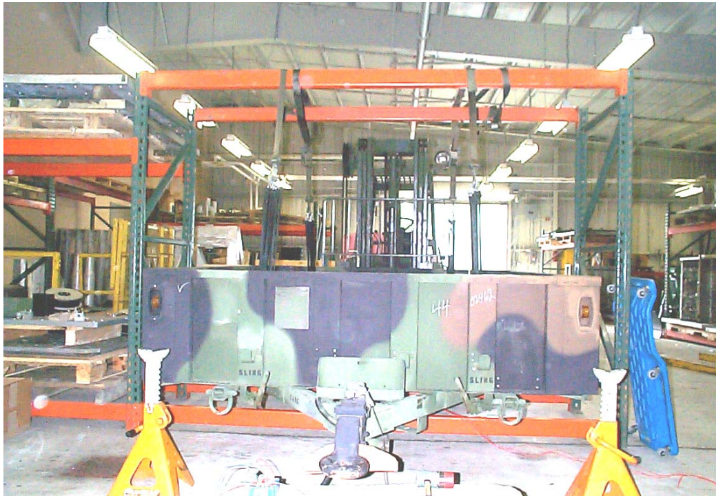
Figure 8: Experimental Modal Analysis Setup Showing Bungee Cord Suspension and Impact Hammer
