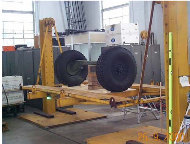
Figure 5: Moment of Inertia Measurement of Wheel and Axle Assembly
