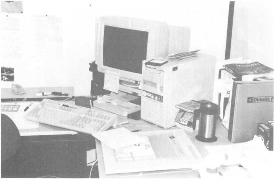
Unsecured computers may fall and suffer damage Photo Credit: Wiss, Janney, Elstner Associates, Inc.
