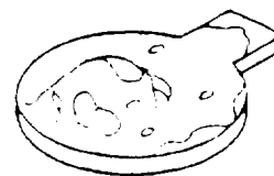
FIGURE 17. Plated-through holes - clinched lead and wires (see 4.19.5.2).
