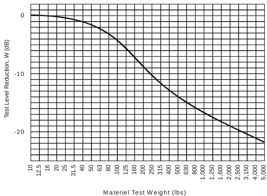
FIGURE 519.5D-5. Test level reduction due to materiel mass loading.
