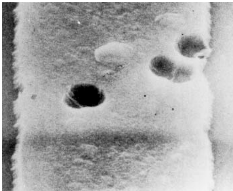
FIGURE 2077-18. (5,000X) General metallization voids (reject).
