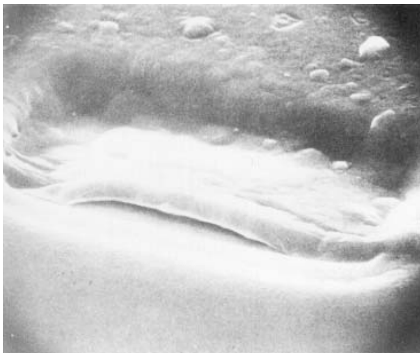
FIGURE 2077-16. (5,000X) Peeling or lifting of general metallization in contact window area (reject).
