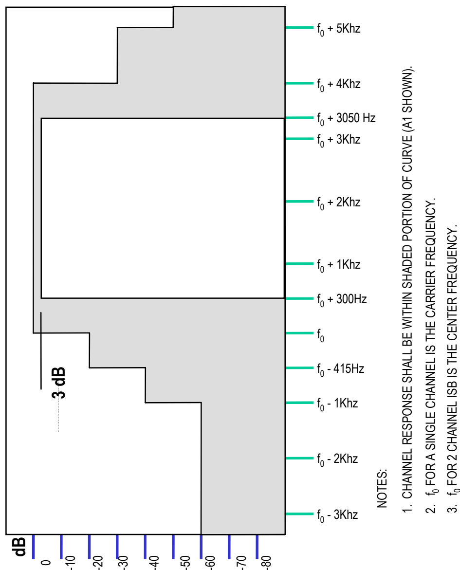
FIGURE 6. Overall channel response for single-channel or dual-channel equipment.
