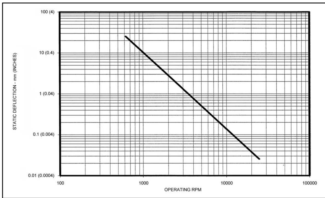
Figure 528-3. Minimum static deflection of mounting for Type II vibration test.
