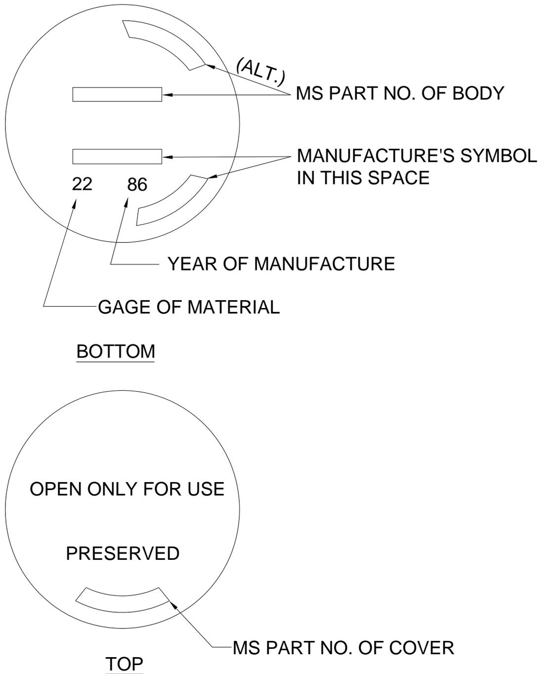
FIGURE 1. DRUM MARKING
