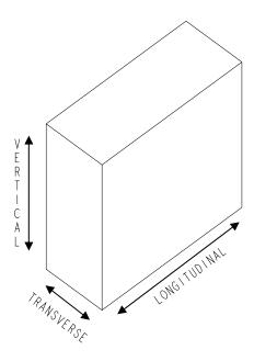
FIGURE 2. Container vibration axes definition
