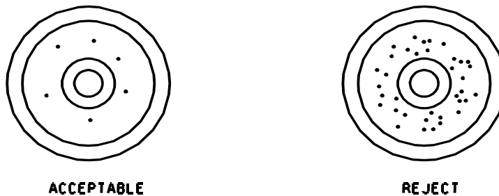
FIGURE A-2. Pinholes.
