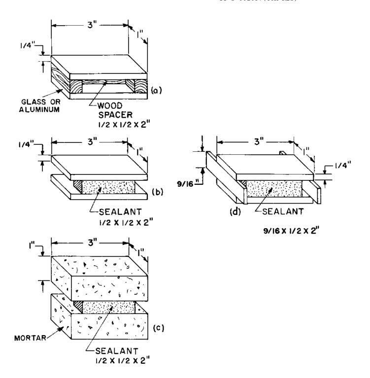
FIG. 8. TEST SPICIMENS IN ENTINSION TEST (a) PREPARED SPICIMEN BEFORE PLACEMENT OF SPALANT, (b) SPALANT WITH SPACERS REMOVED, (c) SPALANT BETWEEN MORTAR BLOCKS, (d) SPALANT IN THE EXTENDED STATE.
