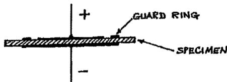
The surface resistance shall be measured by means of a 500-volt megohm bridge exactly 1 minute after the current is applied. Tests following the humidity conditioning shall be made on specimens in the humidity chamber. Surface resistance shall be reported in megohms.
