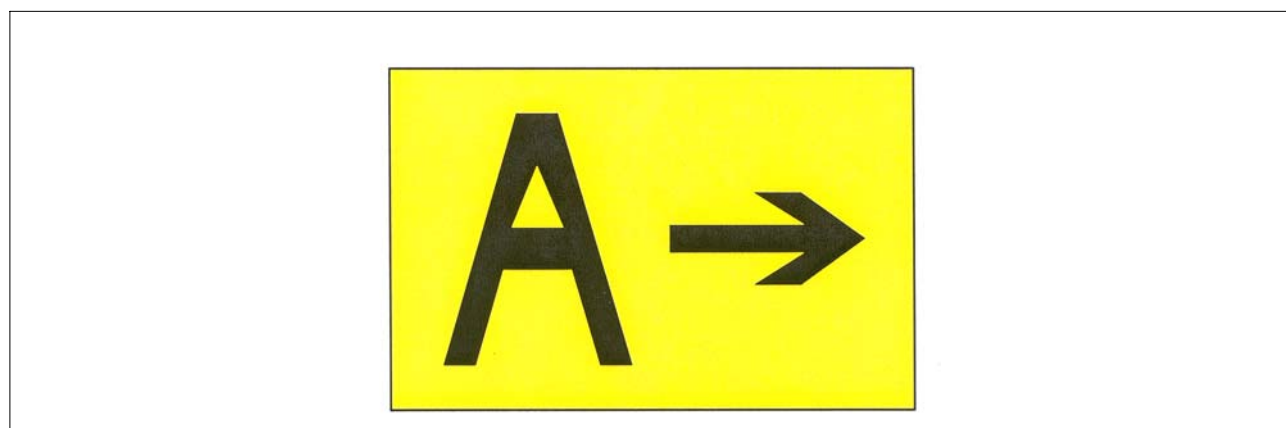
FIG 2-3-36 Direction Sign for Runway Exit
