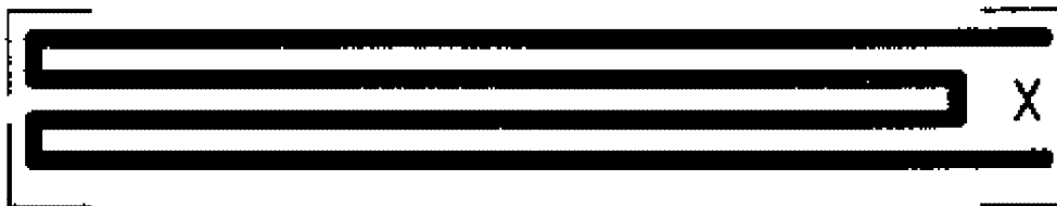
Figure 15: Example of test specimen layout for testing resistance to bending cycles
