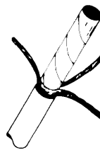
FIGURE 2 GROSS SHIELD PIGTAILS
