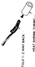
FIGURE 3 TERMINATION OF SPARE CONDUCTORS
