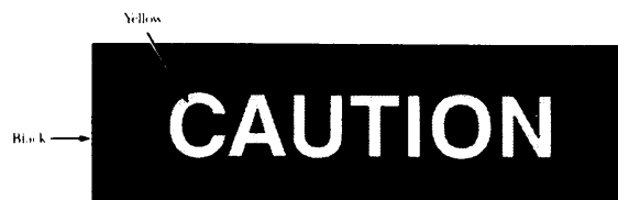
Figure 6-16. Example of a Caution Sign (Ref. 21)
