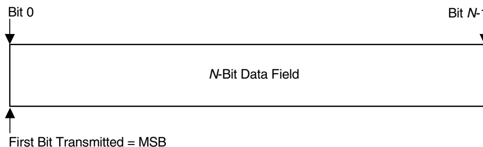
Figure 1-1: Bit Numbering Convention
